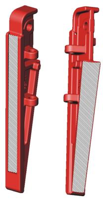
Placing a straight edge against the backs and inside face of the slips will indicate if they are bent or worn. A good slip back is straight, smooth, and well-greased. Slips should be replaced when there is more than 0.062" between the slip back and the straight edge, see below.
