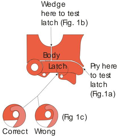
Figure 1: Latch wear inspection
