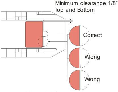
Figure 2: Latch wear inspection
