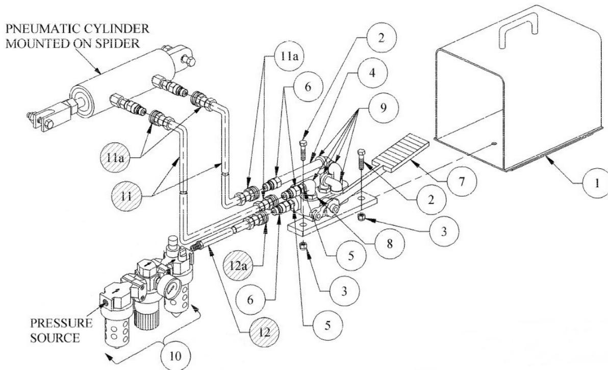
**Figure 3: Foot Operated Pneumatic Control System Assembly**
