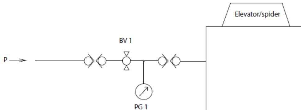
**Figure 1: Pressure test schematic**
